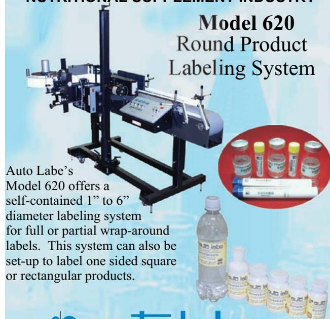
Auto Labe's Model 620 offers a self-contained 1" to 6" diameter labeling system for full or partial wrap-around labels. This system can also be set-up to label one sided square or rectangular products.
